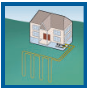
Closed Loop Vertical System
